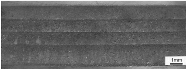
Figure 40. View of the MCMgAl6Zn1 casting magnesium alloy face of weld after laser treatment with TiC, scan rate: 0.75 m/min, laser power: 1.6 kW
